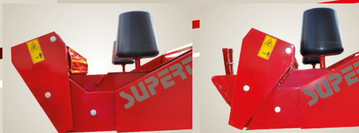
The tilting roller permits wrapping of bales with diameter between 90 and 160 cm.
