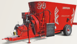
VM3 Twin with double axle balance system with rear steering axle
